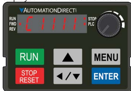
Optional Digital Keypad GS4-KPD Can Display 0~FFFF (hex). (See the 3rd line in the figure below)
