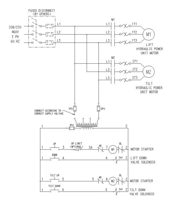
NOTE: UPPER TRAVEL LIMITSWITCH IS OPTIONAL. IF UP LIMIT IS ABSENT, CONNECT WIRE 3 DIRECTLY TO NC CONTACT ON MOTORSTARTER.
